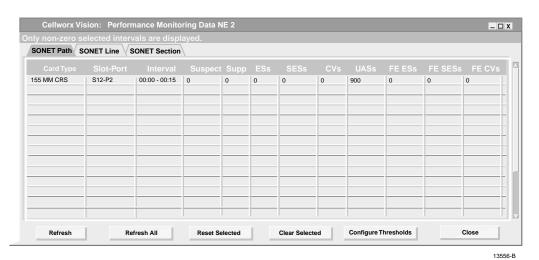
Figure 726-2. Performance Monitoring Data - SONET Port Window
